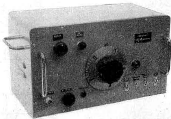
Front view of the Amateur Bands Frequency Meter.
